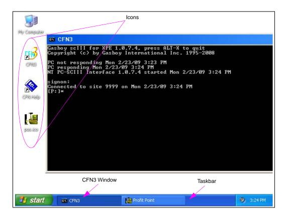
Gasboy is the default login (user) and is the working level of operation. All CFN3 operations occur at this login level. When you turn on the computer the user is Gasboy with GASBOY as the password. The desktop will contain very few icons; CFN3, CFN3 Help, My Computer, and Integral Profit Point (optional). Your day to day site operations use this login.
